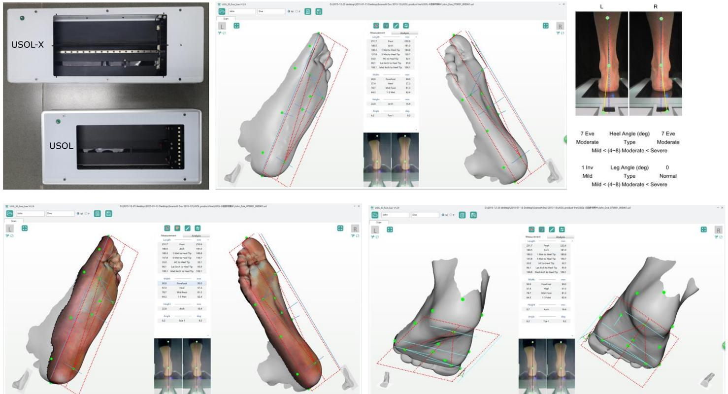
Foot sides scan height up to 80mm; Heel back scan height about 20mm.
